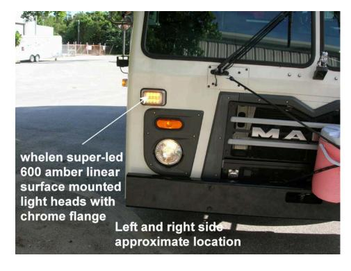
C) Two amber warning side mounted at rear, one right side and one left side flashing amber led emergency flashing lights. These lights will be activated when the vehicle is in reverse and mounted as far to the rear and to the side as possible. Installed no more than 4 foot high as measured from the ground. Whelen vertex style lights are acceptable.
